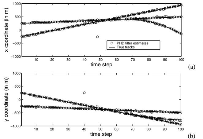
Fig. 3. Position estimates of the Gaussian mixture PHD filter.
