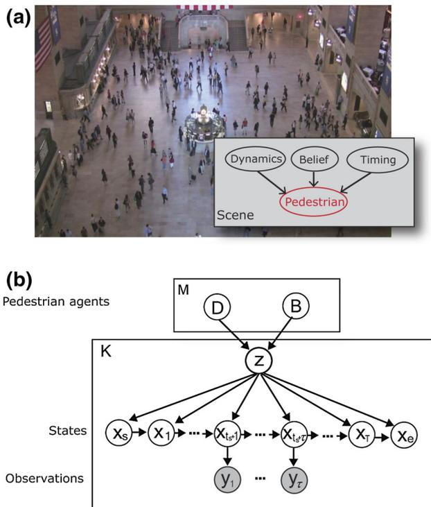
**Fig. 2** (a) The behavior of a pedestrian in crowd is described with three key components, the dynamics of movements, the belief of the starting point and the destination, and the timing of entering the scene. (b) Graphical representation of MDA. The *shadowed* variables are partial observations of the hidden states due to frequent tracking failures in crowded environment
