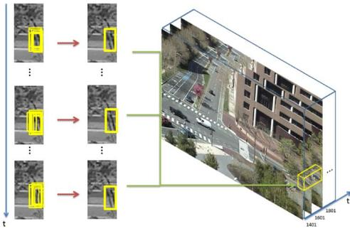
Fig. 5. Hierarchical clustering detection windows in the location-size space. Detection windows in the same frame are first clustered and merged. Merged windows are further clustered across frames. Clusters of detection windows at the same location over a long period are selected as negative samples from the background.
