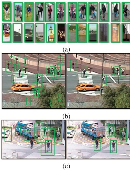
Fig. 1. (a) Positive (first row) and negative (second row) samples from the INRIA data set [4]. (b) Detection results on the MIT Traffic data set and (c) the CUHK Square data set. The left is the results of a generic detector (HOG-SVM [4]) trained on the INRIA data set. The right is the results of a scene-specific detector (also HOG-SVM) automatically trained by our approach.
