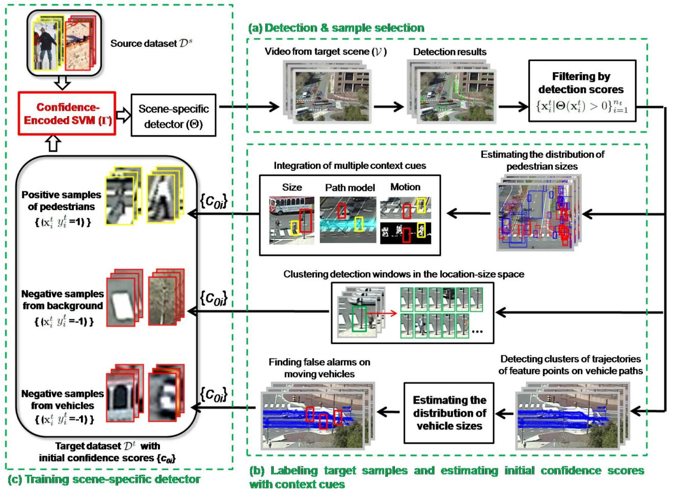
Fig. 2. Diagram of the proposed transfer learning framework. It has three modules: (a) detecting and selecting samples from the target scene, (b) labeling target samples and estimating their initial confidence scores with context cues, and (c) training the scene-specific detectors. Please see the detailed descriptions in Section 1.2.
