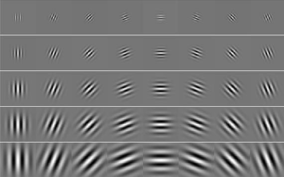
Figure 1. Real part of Gabor kernels at 5 scales and 8 orientations.
