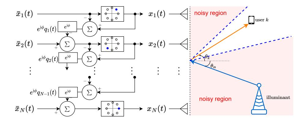
ullet idea: use spatial  $\Sigma\Delta$  mod., with the quantizer being a constant-amplitude discrete-phase rounding function
