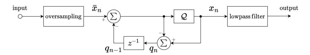
•  $x_n$  is converted to analog via a lowpass filter, which removes much of the q. noise
