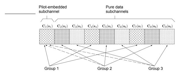
**Fig. 2.** Proposed SG scheme for  $N_c = 9$  and P = 3.
