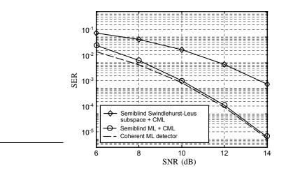
Fig. 5. Performance (SER) comparison to the Swindlehurst-Leus subspace method for Alamouti code, L = 3, P = 8 and  $N_r = 6$ .
