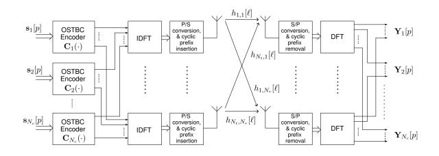
Fig. 1. OSTBC-OFDM system structure diagram.
