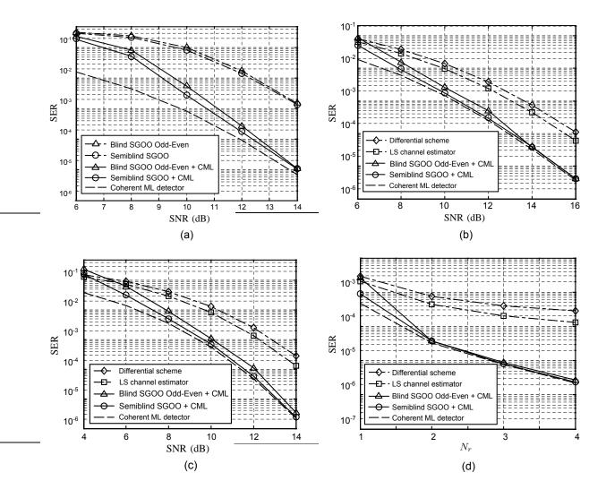
Fig. 3. Performance (SER) of the proposed schemes for QPSK  $4 \times 3$  OSTBC, P = 16, (a) L = 12 and  $N_r = 3$ , (b) L = 8 and  $N_r = 2$ , (c) L = 8 and  $N_r = 4$ , (d) L = 8 and SNR= 14 dB.
