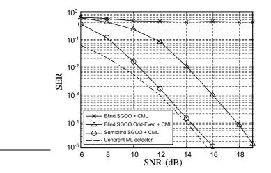
Fig. 4. Performance (SER) of the proposed schemes for QPSK Alamouti code, P = 8, L = 8 and  $N_r = 4$ .
