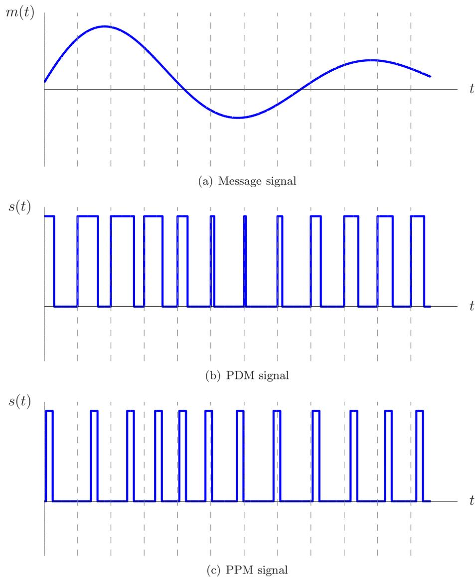
Figure 2: A waveform illustration of PDM and PPM. The grey vertical lines mark the sampling time instants.
