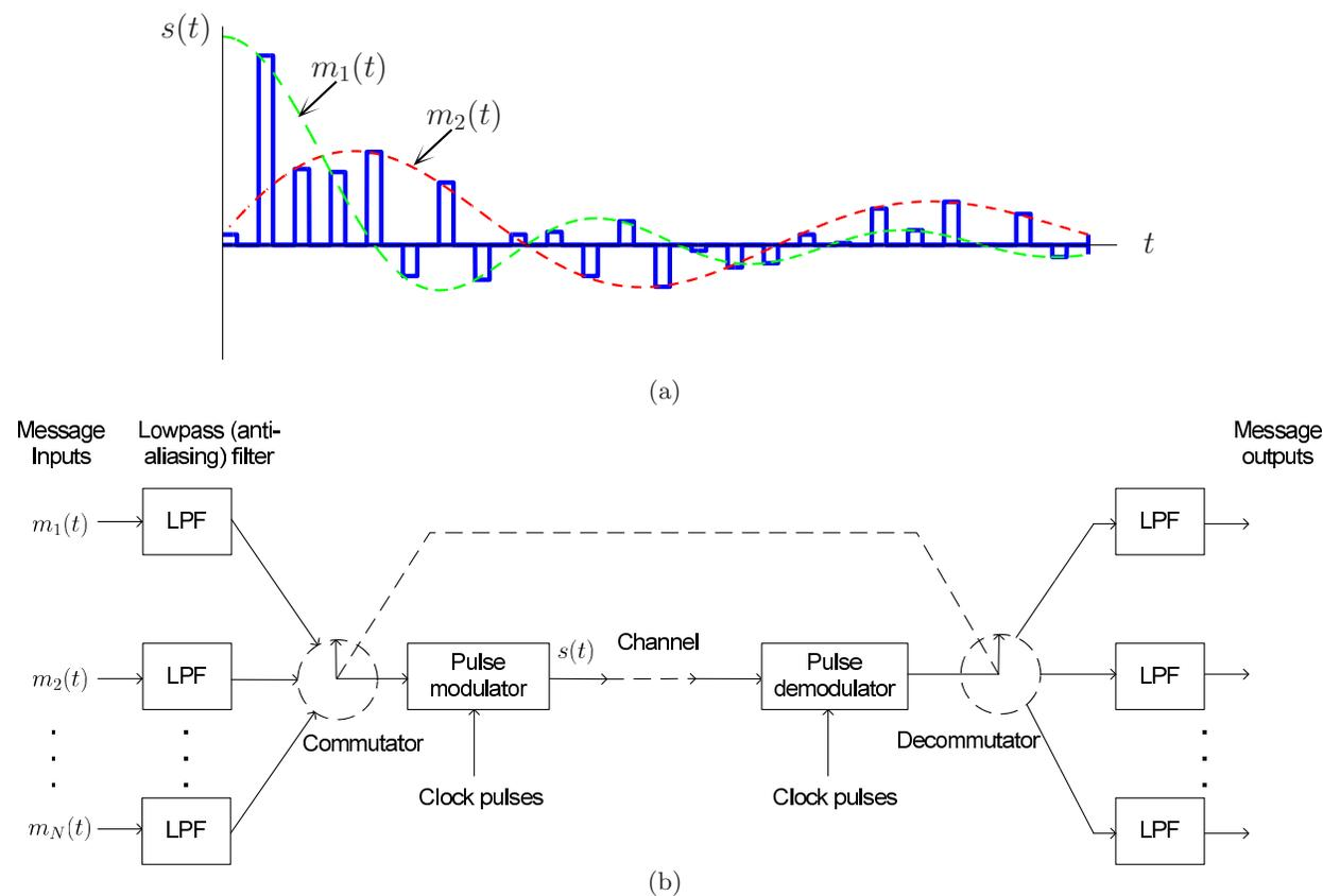
Figure 6: Time division multiplexing. (a) An illustration of the TDM signal for the case of two message signals. (b) An TDM system diagram.
