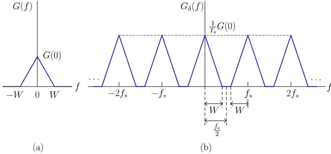
Figure 4: Illustration of the spectrum of  $g_\delta(t)$ .
