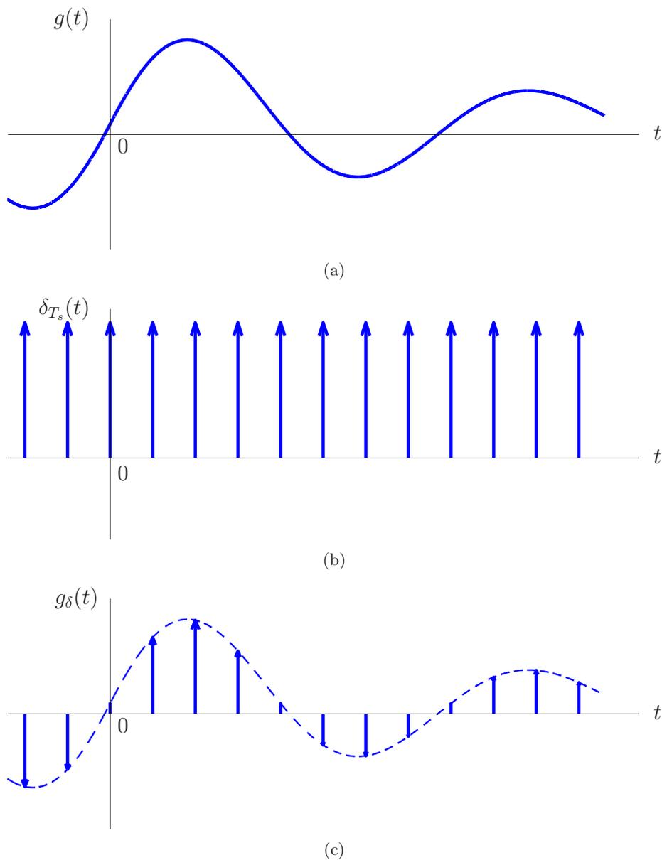
Figure 3: A waveform illustration of the sampling process.
