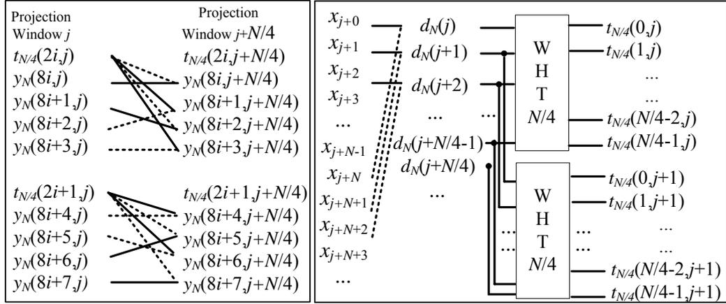
Fig. 3 Signal flow diagram of the bottom up algorithm for order- $N$  sequency WHT
