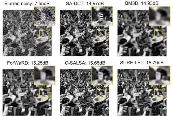
Fig. 7. Restoration of *Crowd* degraded by Gaussian blur of variance 9 with noise std  $\sigma = 100$ .
