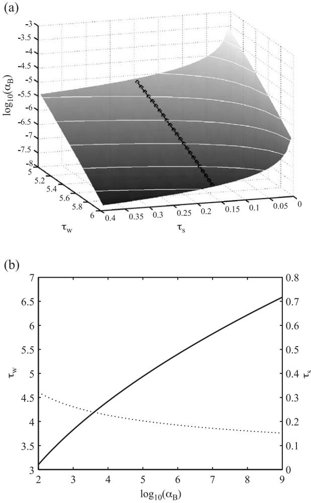
Fig. 4. Simplified case where  $\sigma_k$  is assumed to be known. (a) Probability surface. Equiprobable contour lines are in white. The circular dots mark the optimal threshold values. (b) The optimal threshold values  $\tau_w$  (full line) and  $\tau_s$  (dotted line).
