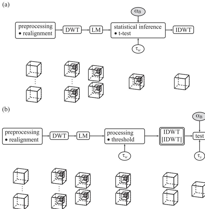
Fig. 2. (a) The standard wavelet-based approach. The desired significance level  $\alpha_B$  is fed to the statistical inference stage in the wavelet domain. (b) The approach of the present paper is to reinterpret the wavelet threshold as a general algorithm parameter. After reconstruction, a statistical test is performed in the spatial domain, taking into account the wavelet processing.
