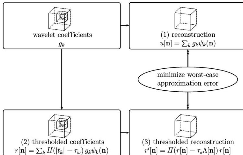
Fig. 5. Principle of minimizing the worst-case approximation error between the detected and the unprocessed parameter map, represented by  $r'[\mathbf{n}]$  and  $u[\mathbf{n}]$ , respectively.
