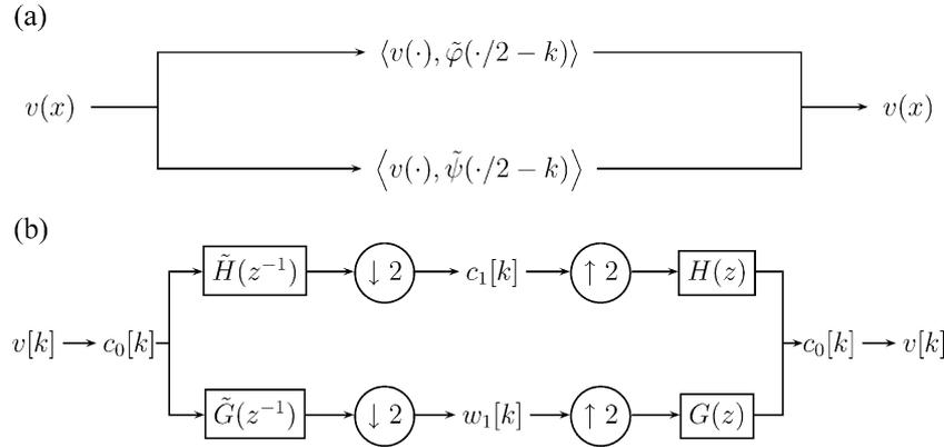
Fig. 1. The discrete wavelet transform for one iteration. (a) The continuous-domain representation. (b) The filterbank representation.
