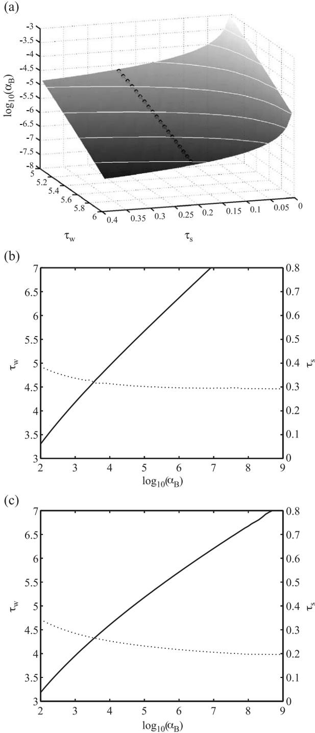
Fig. 6. General case taking into account the estimate of  $\sigma_k$ . (a) Probability map. The white contour lines are equiprobable. The circular dots mark the optimal threshold values. (b) Optimal threshold values for  $N_t = 50$ . (c) Optimal threshold values for  $N_t = 150$ .
