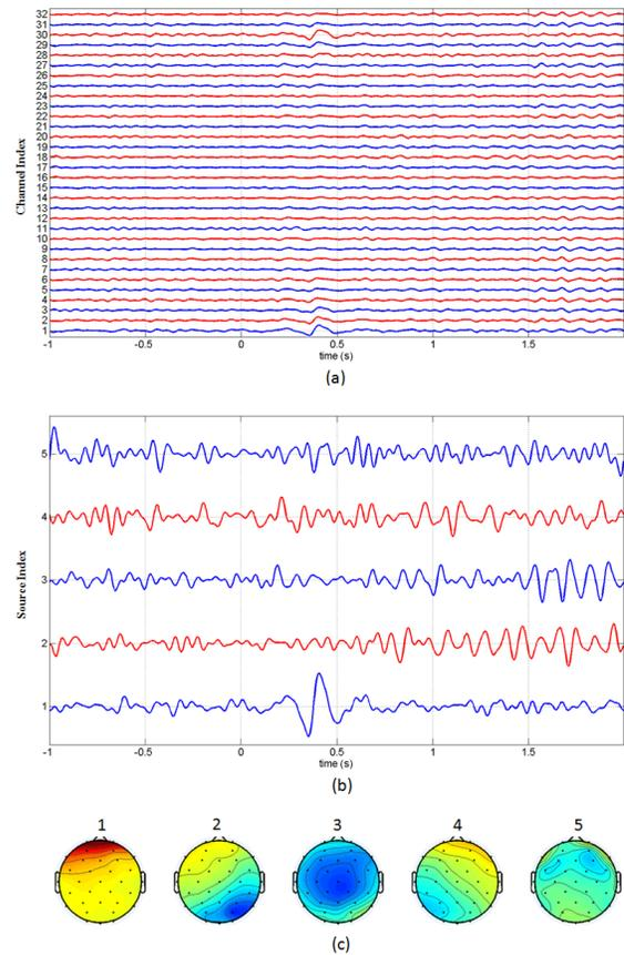
Fig. 3. Illustration of (a) Electrode plots of one single-trial raw EEG recordings, around 0.4s there was a clear eye artifact. (b) The time course of the separated source and (c) The topographies of the separated source.
