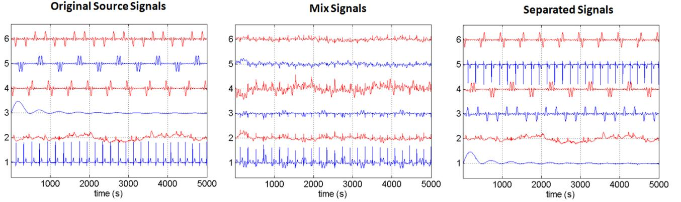
Fig. 1. Illustration of Blind Source Separation based on Weak Exclusion Principle (WEP) Using Simulated Data.
