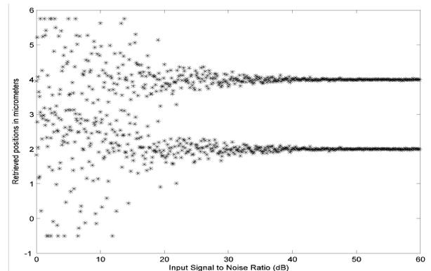
Fig. 2: Retrieved positions of the interfaces as a function of the input noise: for SNR>20dB, the two layers can be separated.
