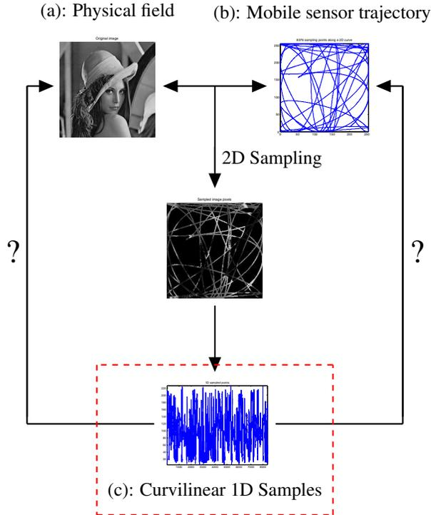
**Fig. 1:** Our goal (“FRI sensing”) is to reconstruct the physical field (a) and the sampling trajectory (b) of the mobile sensor from the measured curvilinear 1D time samples (c) (framed by a red box).
