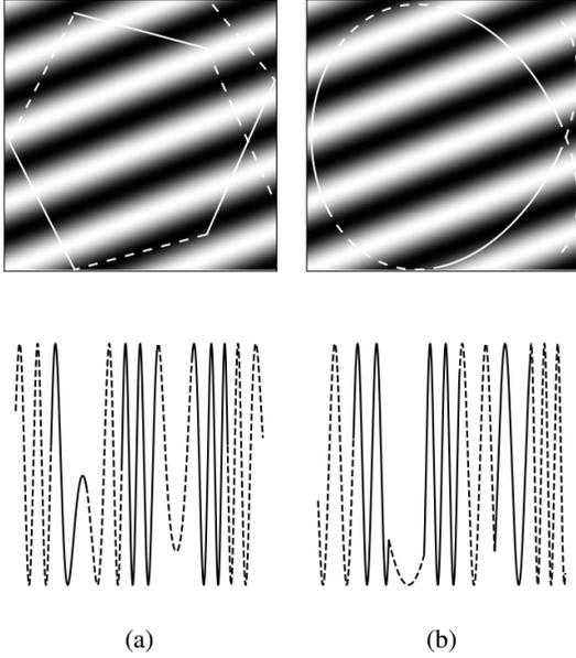
**Fig. 2:** (a) Sampling a sum of spatial sinusoids along straight line segments results in an exact piecewise sinusoidal 1D signal. (b) Sampling the same image along a curved trajectory with small curvature results in an approximate piecewise sinusoidal 1D signal.
