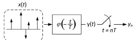
**Fig. 1.** The FRI acquisition system. The continuous-time input signal  $x(t)$ , in this case a sequence of  $K$  Diracs, is filtered by a sampling kernel  $\varphi(-t/T)$  and sampled at a period  $T$ .
