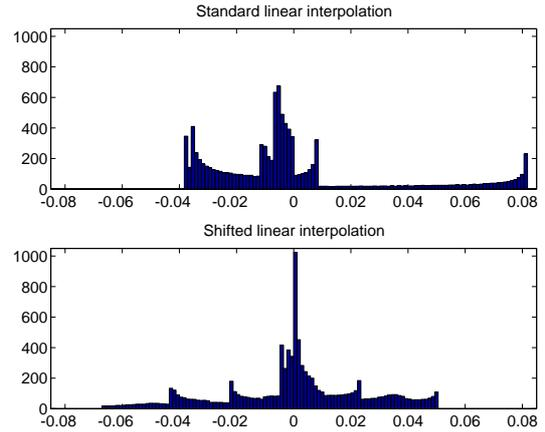
**Fig. 4.** Optimally-shifted versus standard linear interpolation: comparison of the error histograms—counts of the values of  $(f(x) - f_T(x))$ —resulting from the interpolation of the function of Fig. 1. Notice the strong dissymmetrical distribution of the errors in the standard method.
