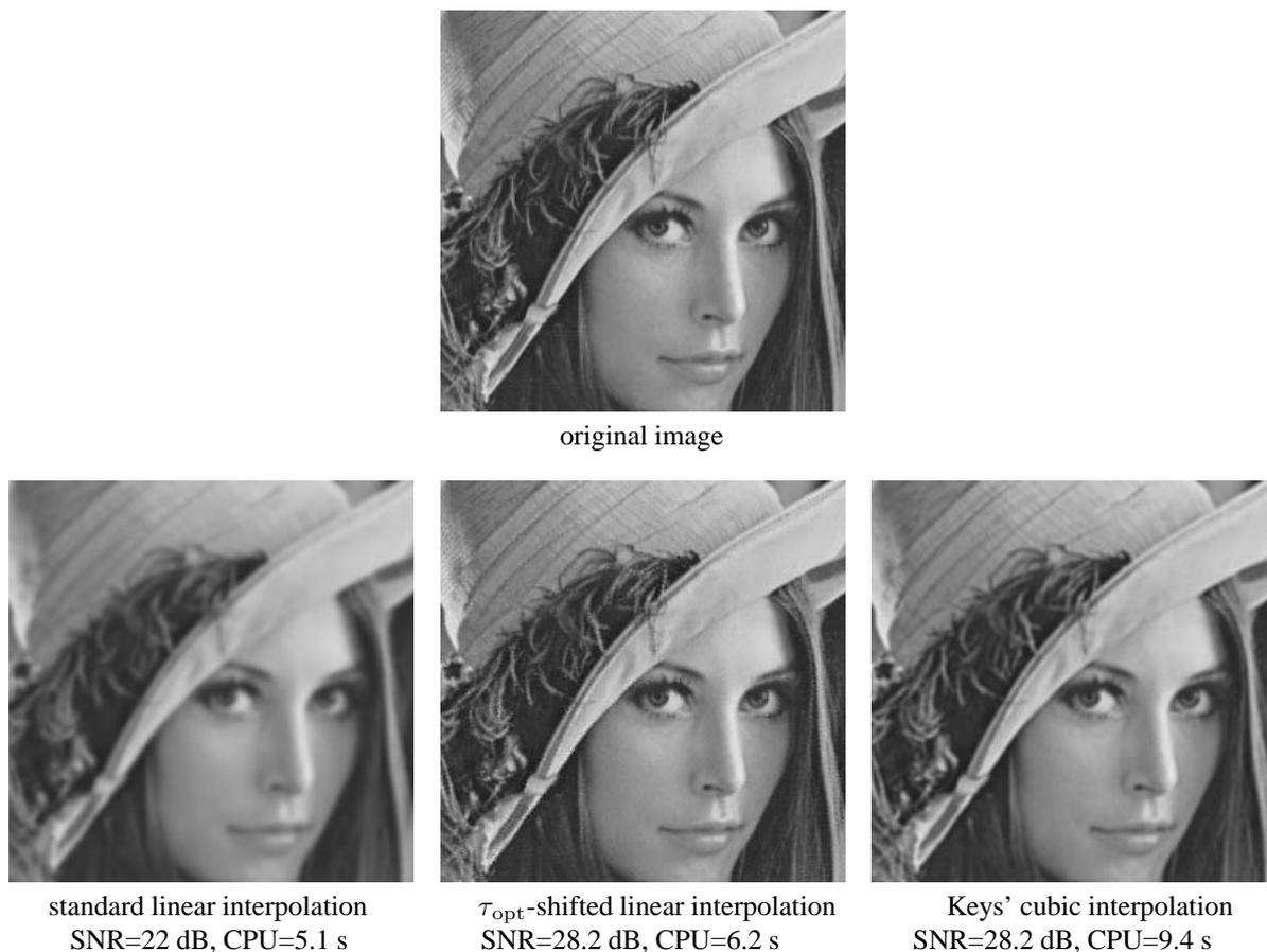
**Fig. 5.** 15 successive rotations by  $24^\circ$  of Lena using standard, shifted linear, and Keys' interpolations: Notice the sharpness of the shifted method, as compared to the two others.
