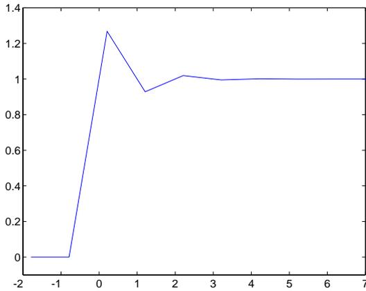
**Fig. 3.** Gibbs phenomenon caused by the—optimally—shifted linear interpolation of a unit step function.
