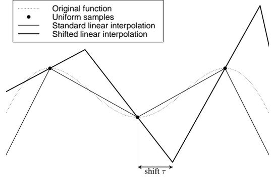
**Fig. 1.** “Shifted” versus “standard” linear interpolation; here,  $\tau = 0.4$  which is far from the optimum (8).
