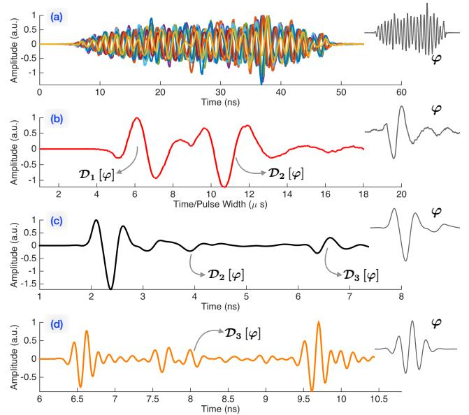
**Fig. 1:** Disparate case studies where the measurements are delayed, amplitude-scaled and distorted versions of the reference pulse  $\varphi$  shown in the inset. (a) Free electron laser measurements in Electron Paramagnetic Resonance. (b) Photoacoustic imaging. (c) Ground penetrating radar. (d) Ultra-wide band array.
