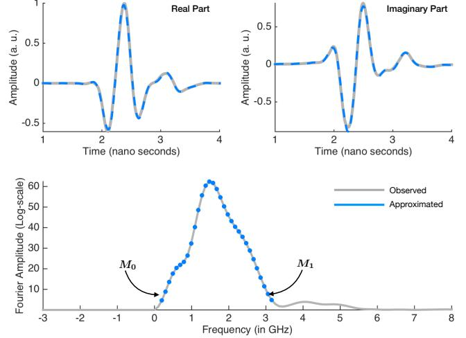
**Fig. 3:** Approximation of kernel used for ground penetrating radar experiment via finite Fourier series. The measured data is shown in grey ink. Dashed blue lines show its approximated version. Here  $T = 10.14$  ns and  $M_0 = 0.19$  GHz and  $M_1 = 3.15$  GHz.
