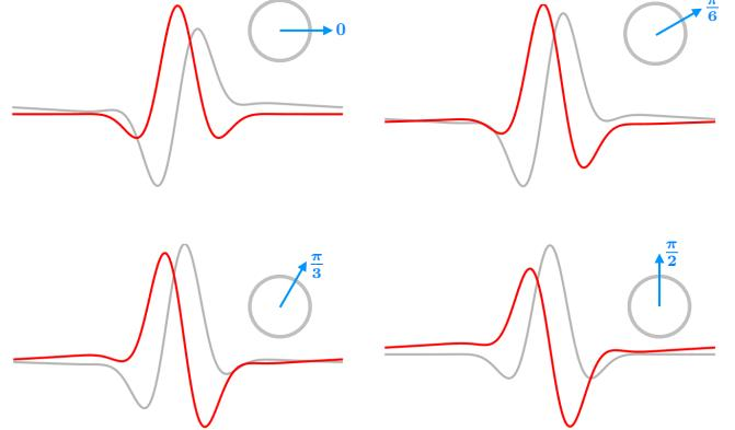
Fig. 2: We plot real (red) and imaginary (grey) parts of pulse  $e^{j\theta_k}\varphi(t)$ ,  $\theta_k = \pi k/6$ ,  $k = 0, \dots, 4$  where  $\varphi$  is chosen to be a modulated Gaussian function (Gabor window) such that the real and imaginary parts form a quadrature pair.
