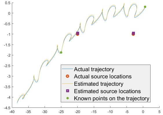
**Fig. 3:** Actual and reconstructed trajectory and source locations (reconstruction shifted by 0.05 for visualisation purposes), in the case in which the activation times of the sources are unknown, and we know the locations of two sample points.
