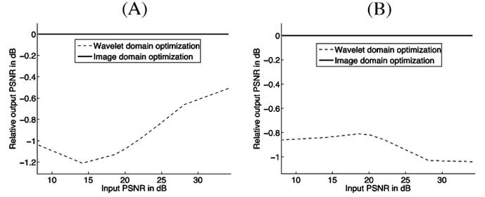
Fig. 3. Comparison of the proposed *SURE-LET* denoising procedure with a SURE-based denoising algorithm optimized in the wavelet domain when using the undecimated wavelet (*Haar*) transform: (a) *House*; (b) *Al*.
