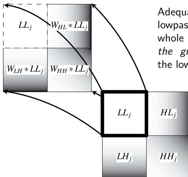
Adequate high-pass filtering of the lowpass  $LL_j$  — which contains the whole parent tree:  $W$  compensates the *group-delay* difference between the low-pass and the high-pass band.
