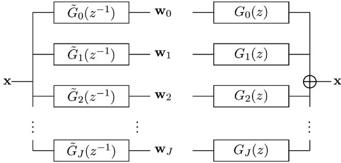
Fig. 1. Undecimated  $J$ -band analysis-synthesis filterbank.
