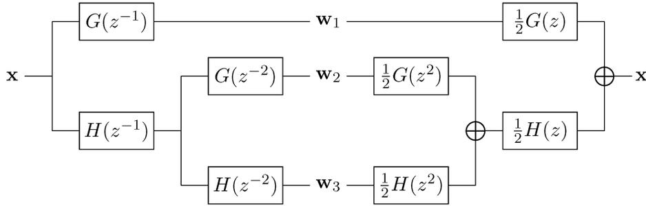
Fig. 2. Classical undecimated wavelet filterbank for 1-D signal.
