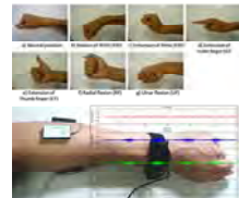
Targeted 6 hand gestures, assignment of surface electrodes and their signals
