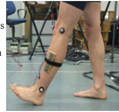
Measuring Segment Orientation with the Developed Device
