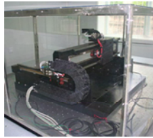
Experimental Testbed - An Industrial Precision Gantry System
