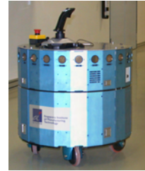
Omnidirectional wheeled mobile robot developed in SIMTech
