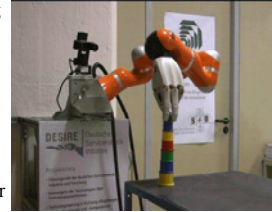
SAHand mounted on Kuka LBR Arm building up a tower with toy cups
