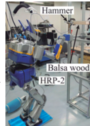
Nailing task by HRP-2
