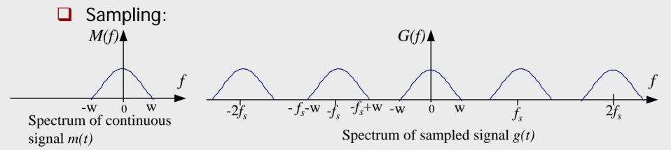
Nyquist's criterion: the minimum sampling rate needed to avoid loss of information in a signal which is band-limited to a bandwidth of w is 2w.
