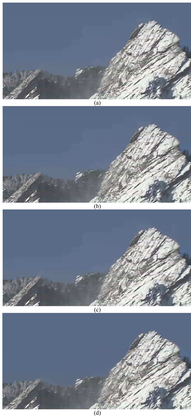
Fig. 13. Frame 3 of (a) Input H.264/AVC decompressed video (CR = 3347 : 1) with contour artifacts, MADAI = 0.7821; (b) result of Bhagavathy et al. [18] using original settings, MAMDAI = 0.9242; (c) result of Yoo et al. [19], MADAI = 0.7087; (d) result of the proposed decontouring method, MADAI = 0.3376. MADAI of the uncompressed frame equals to 0.1556.
