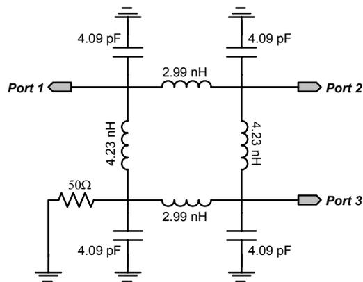
Fig. 2. The schematic of the lumped element 3-dB hybrid coupler with center frequency of 1.88GHz.
