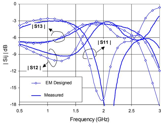
Fig.4. The measured and the EM designed performance of the LTCC lumped element 3-dB hybrid coupler.
