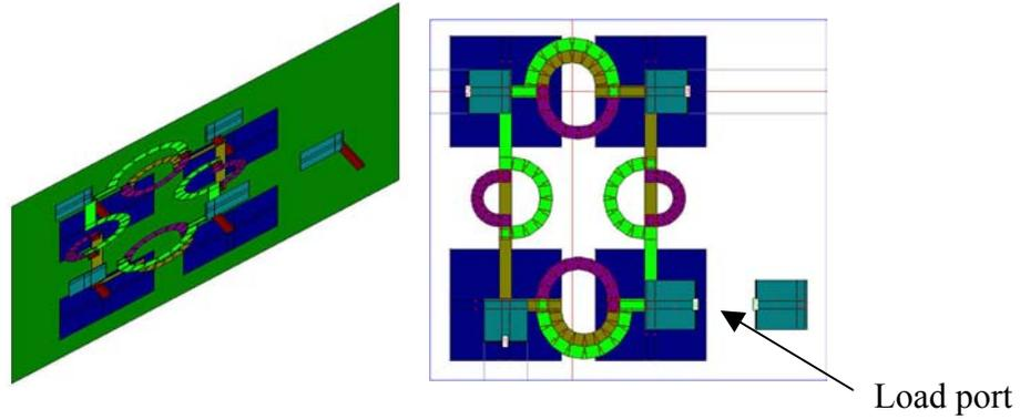
Fig.3. The top and perspective views of the layout of the lumped element coupler in a 7-layer LTCC substrate.
