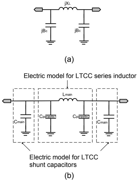
Fig.1. (a) A low-pass ‘ $\pi$ ’ network for replacing quarter wavelength transmission line. (b) The ‘ $\pi$ ’ network with possible parasitic capacitance.
