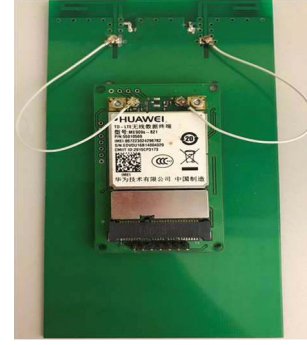
Fig. 4. Connection of two MIMO antennas with a TD-LTE data communication module for experimental validation.
