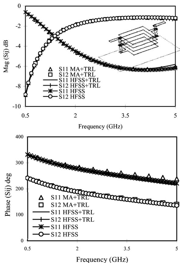
Fig. 4.  $S$ -parameters of a multilayer capacitor defined at the device ports.
