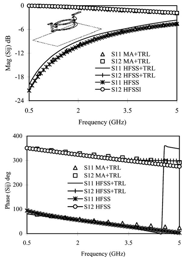
Fig. 3.  $S$ -parameters of a spiral inductor defined at the device ports.
