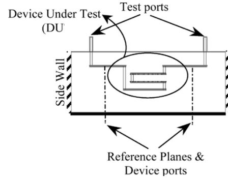
Fig. 1. Side view of the model for modal analysis for a multilayered passive circuit and the definitions of test ports and device ports.
