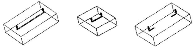
Fig. 2. Perspective view of TRL calibration standards.
