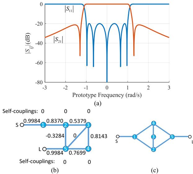
Fig. 5. (a) Symmetric response of a 5-2 filter in the low-pass domain. (b) Normalized seed coupling matrix in folded form. (c) Legitimate coupling topology with redundancy.
