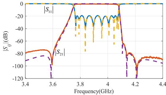
Fig. 11. Synthesized and measured responses (solid lines refer to the synthesized and dashed lines refer to the measured) of the prototyped 9-4 filter in the  $3 \times 3$  grid configuration.
