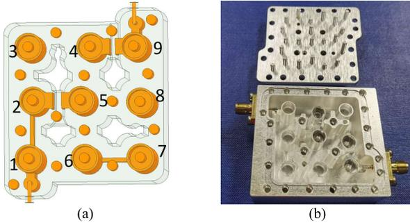
Fig. 10. Prototyped 9-4 filter in the  $3 \times 3$  grid configuration using combine resonators. (a) Internal model for EM design. (b) Photograph of the prototyped 9-4 filter (inner dimensions:  $40 \times 40 \times 15 \text{ mm}^3$ ).
