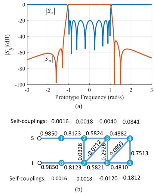
Fig. 6. (a) Asymmetric response of an 8-4 filter. (b) Normalized seed coupling matrix in folded form.
