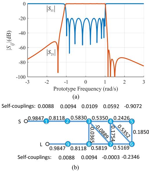
Fig. 8. (a) Asymmetric response of the 9-4 filter. (b) Normalized seed coupling matrix in folded form of the 9-4 filter.
