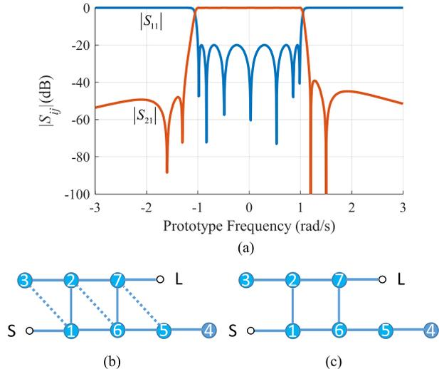
Fig. 4. (a) Asymmetric response of a 7-4 filter in the low-pass domain. (b) Target coupling topology that satisfies the  $N_M = N_F$  condition. (c) Coupling topology with an approximate solution in the cul-de-sac topology.
