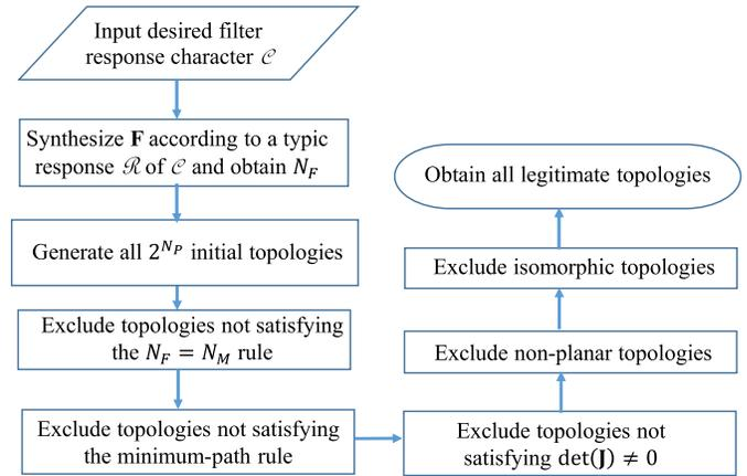
Fig. 2. Flowchart of exhaustive search process for legitimate coupling topologies.
