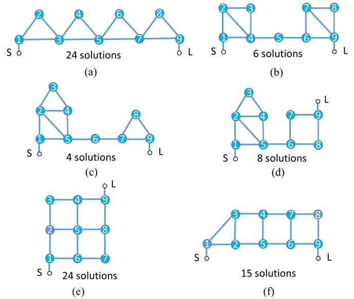
Fig. 9. Some of the coupling topologies for the 9-4 filter. (a) Cascaded tri-section. (b) Cascaded quadruplet. (c) Cascaded quintet- and tri-section. (d) Cascaded quintet and box sections. (e) “Grid” configuration. (f) “Trapezoid” configuration.
