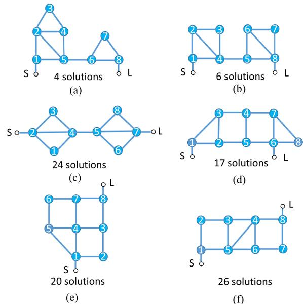
Fig. 7. Some of coupling topologies for the 8-4 filter response. (a) Cascaded quintet- and tri-section. (b) Cascaded quadruplet sections. (c) Two cascaded modified quadruplets. (d) "Trapezoid" configuration. (e) "Grid" configuration. (f) "Full-box" configuration.
