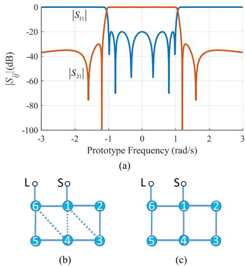
Fig. 3. (a) Symmetrical response of a 6-4 filter in the low-pass domain. (b) Target coupling topology for the 6-4 filter. (c) Coupling topology for the 6-4 filter in the Pfitzenmaier topology.
