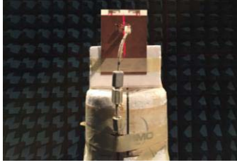
Fig. 10. Measurement setup for antenna radiation pattern and total efficiency.
