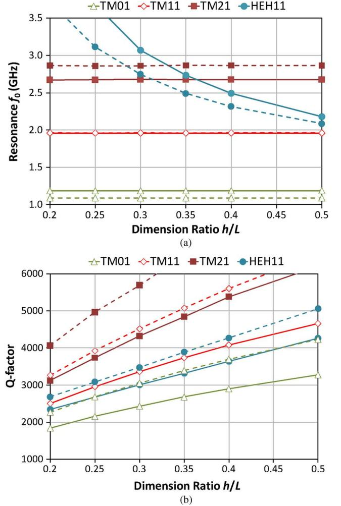
Fig. 5. First four modes of a short-circuited dielectric resonator with  $d$  and  $L$  fixed,  $h$  varies: (a) resonance frequencies and (b)  $Q$  factors. The solid lines are for the resonator with  $d = 28.8$  mm,  $L = 41$  mm, and the dashed lines are for the resonator with  $d = 32.4$  mm,  $L = 50$  mm.
