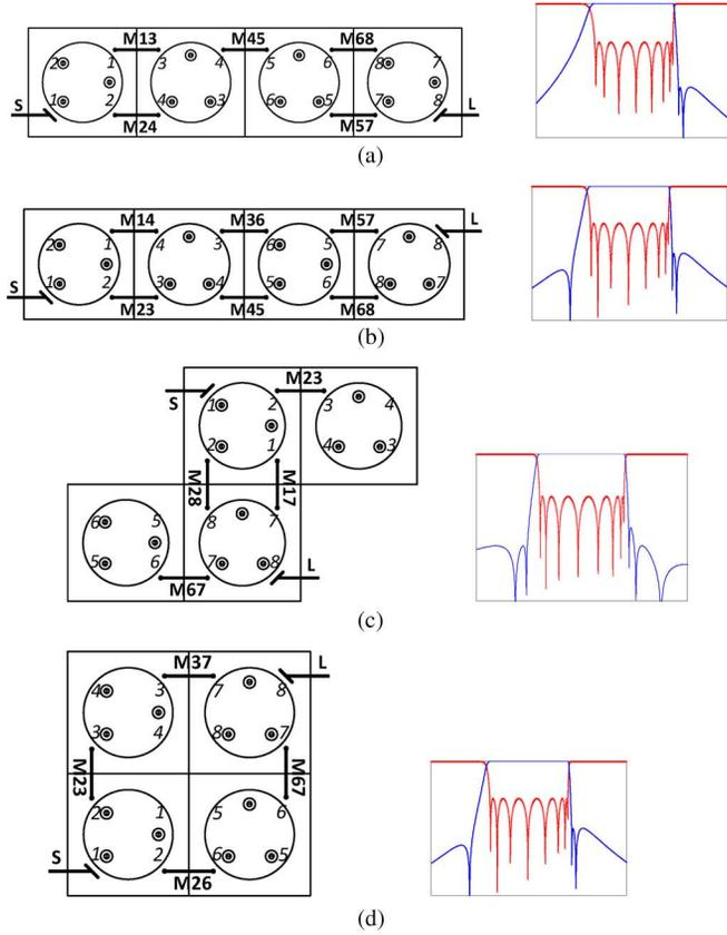
Fig. 12. Eighth-order asymmetric filter coupling configurations and their ideal responses for the proposed  $TM_{11}$  dielectric resonators. (a) Box. (b) Extended-box. (c) Cul-de-Sac. (d) Further Cul-de-Sac.
