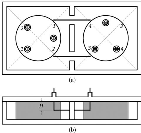
Fig. 10.  $TM_{11}$  dielectric resonator filter with the alternative inter-cavity coupling loops. (a) Top view. (b) Side view.
