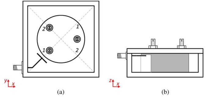
Fig. 8. Grounded strip loop structure for I/O coupling of a dual  $TM_{11}$  mode filter. (a) Top view of an end cavity. (b) Side view of the I/O coupling structure.
