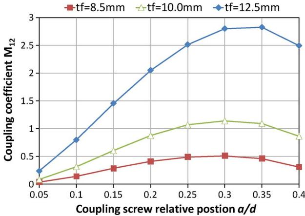
Fig. 7.  $TM_{11}$  degenerate mode coupling coefficient  $M_{12}$  change with the screw relative positions and penetration depths.
