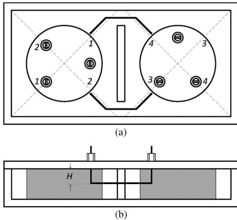
Fig. 9.  $TM_{11}$  dielectric resonator filter with V-shape inter-cavity coupling loops. (a) Top view. (b) Side view.
