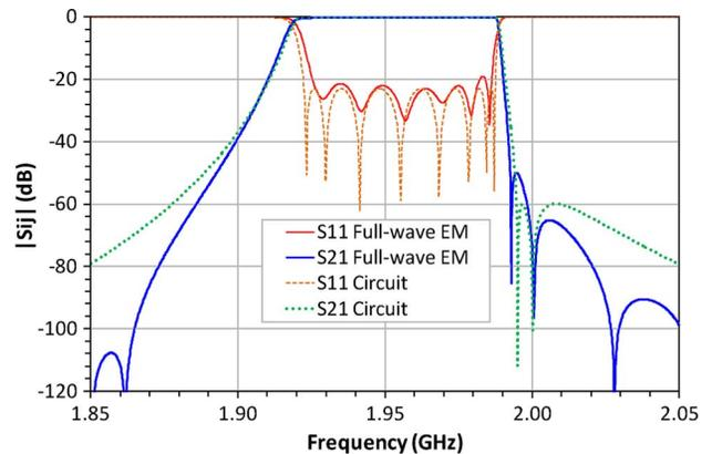
Fig. 18.  $S$ -parameters comparison between the full-wave EM model and the circuit model of the eight-pole asymmetric filter in *box* coupling topology.
