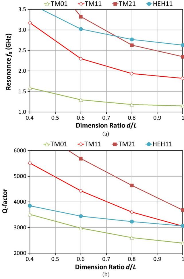
Fig. 4. First four modes of a short-circuited dielectric rod in a fixed  $L = 41$  mm,  $h = 14$  mm cavity with the change of  $d$ . (a) Resonance frequencies. (b)  $Q$  factors.
