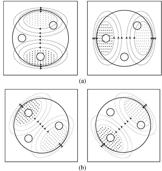
Fig. 3. EM field modal plot (top view) of the  $TM_{11}$  degenerate modes in a resonator with the: (a) coupling hole on the cavity diagonal and (b) coupling hole on the horizontal axis. (left)  $v$  mode. (right)  $h$  mode. Dashed lines:  $H$ -field. Dots and crosses:  $E$ -field.
