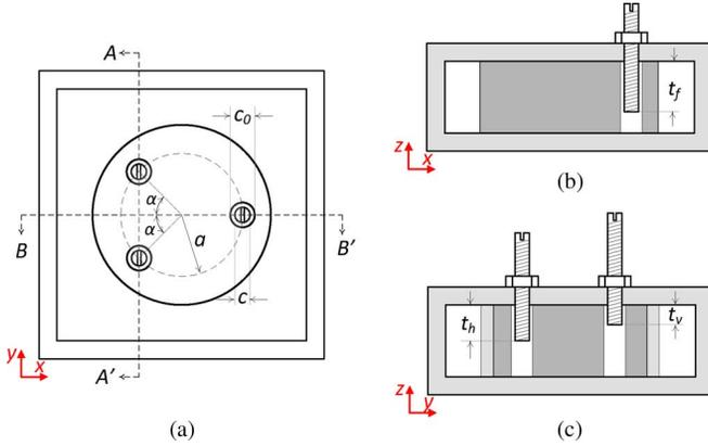
Fig. 6. TM dual-mode resonator degenerate mode tuning and coupling structure with key dimension parameters. (a) Top view. (b)  $BB'$  cross-section view. (c)  $AA'$  cross-section view.
