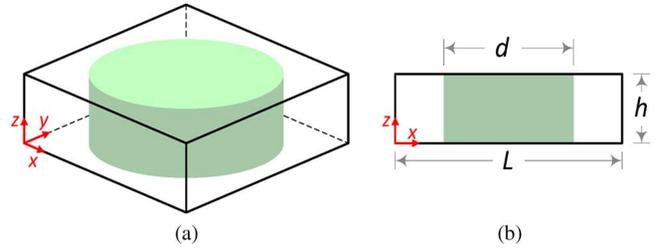
Fig. 2. Resonator with dielectric rod short-circuited to the metallic cavity walls. (a) 3-D view and (b) cross-section view with dimension parameters.
