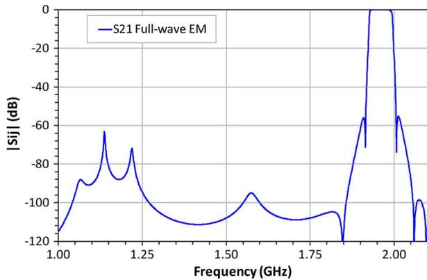
Fig. 16.  $S_{21}$  curve of the  $TM_{11}$  dielectric resonator filter with lower spurious  $TM_{01}$  mode suppressed.
