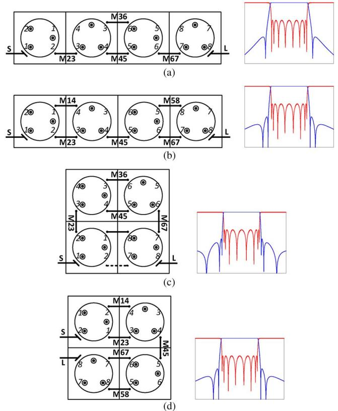
Fig. 11. Eighth-order symmetric filter coupling configurations and their ideal responses with the proposed  $TM_{11}$  dual-mode dielectric resonators. (a) *Folded* in straight-line layout. (b) *CQ* in straight-line layout. (c) *Folded* in folded-line layout. (d) *CQ* in folded-line layout.
