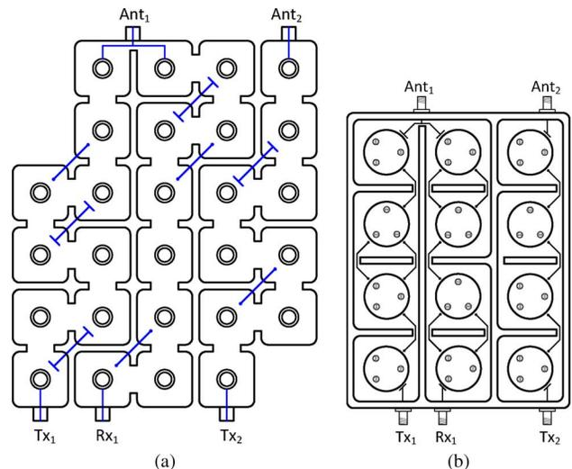
Fig. 1. Planar-coupled filter/diplexer configuration: (a) by conventional single mode coaxial resonators and (b) by the proposed dual-mode  $TM_{11}$  dielectric resonators.
