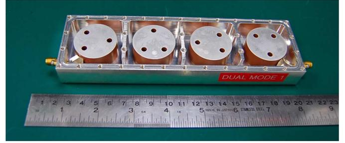
Fig. 13. Photograph of the prototyped eight-pole  $TM_{11}$  dual-mode dielectric resonator filter hardware with upper lid removed.
