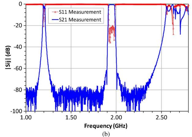
Fig. 14. Measured result of the eight-pole  $TM_{11}$  dual-mode dielectric resonator filter. (a) In-band  $S$ -parameters responses. (b) Broadband  $S$ -parameters responses.
