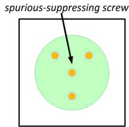
Fig. 15. Top view of the  $TM_{11}$  dielectric resonator with  $TM_{01}$  spurious mode suppression screw in the center.
