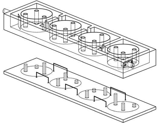
Fig. 17. Full-wave EM model of the eight-pole  $TM_{11}$  dielectric resonator filter in *box* coupling topology.
