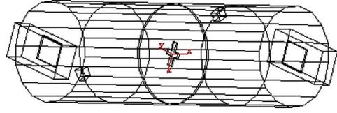
Fig. 3. Four-pole circular waveguide dual-mode filter.
