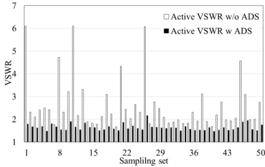
Fig. 9. Worst active reflection coefficients among the antenna ports of the eight-element array in frequency band of 50 MHz in 50 random sets of ZF precoding weighting coefficients.
