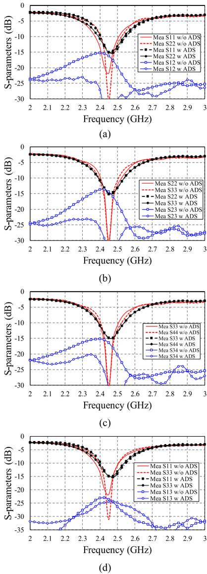
Fig. 7. Representative measured S-parameters of the eight-element air patch array with and without the ADS of (a) antennas 1 and 2, (b) antennas 2 and 3, (c) antennas 3 and 4, and (d) antennas 1 and 3.
