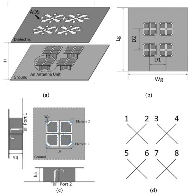
Fig. 11. 2 by 2 dual-polarized dipole array. (a) Perspective view of the array with the ADS. (b) Top view of the array. (c) Top and side views of one antenna unit consisting of two dual-polarized antenna elements. (d) Number assignment of the eight antenna elements.
