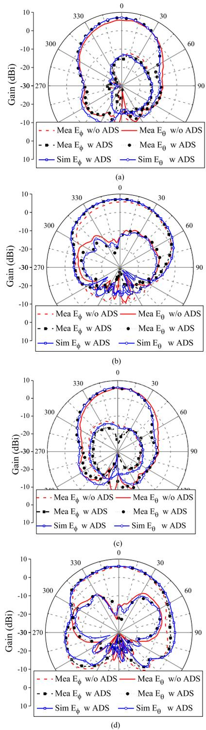
Fig. 8. Representative radiation patterns of the eight-element air patch array with and without the ADS. (a) E-plane patterns of element 1. (b) H-plane patterns of element 1. (c) E-plane patterns of element 3. (d) H-plane patterns of element 3.
