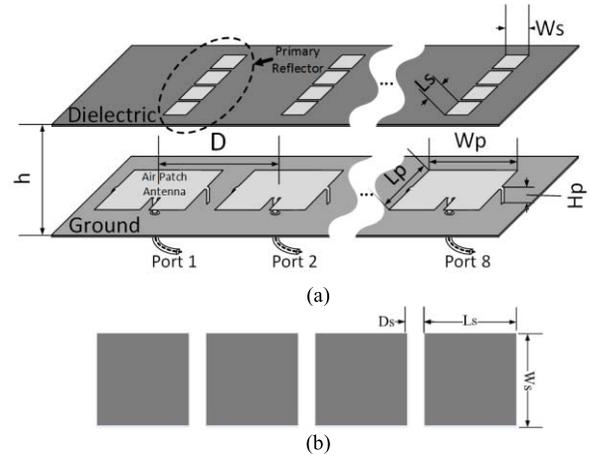
Fig. 3. (a) Eight-element linearly polarized air patch array antenna and an ADS with eight metal broken strips. (b) Dimensions of a metal broken strip.
