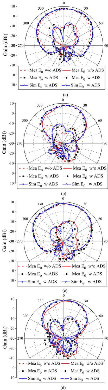
Fig. 15. Representative radiation patterns of the 2 by 2 dual-polarized dipole array with and without the ADS. (a) H-plane patterns of element 1. (b) E-plane patterns of element 1. (c) H-plane patterns of element 2. (d) E-plane patterns of element 2.
