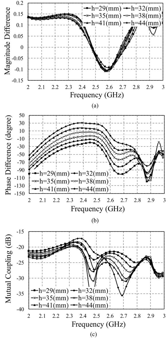
Fig. 4. Simulated (a) magnitude difference, (b) phase difference, and (c) mutual coupling with different heights and  $W_s = 15$  mm and  $D_s = 1$  mm.
