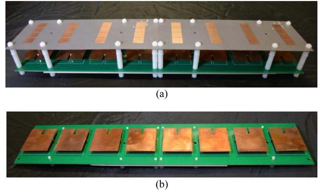
Fig. 6. Photograph of the prototype of (a) eight-element linear air patch array with the ADS and (b) array without the ADS.
