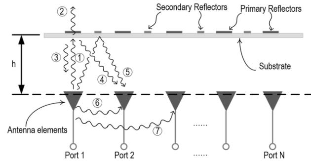
Fig. 1. Schematic of an array antenna and an ADS with spacing distance  $h$ .
