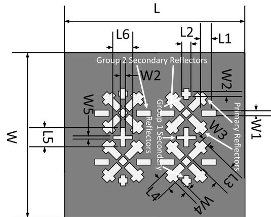
Fig. 12. Metal reflection patches on the ADS for the 2 by 2 dipole array.
