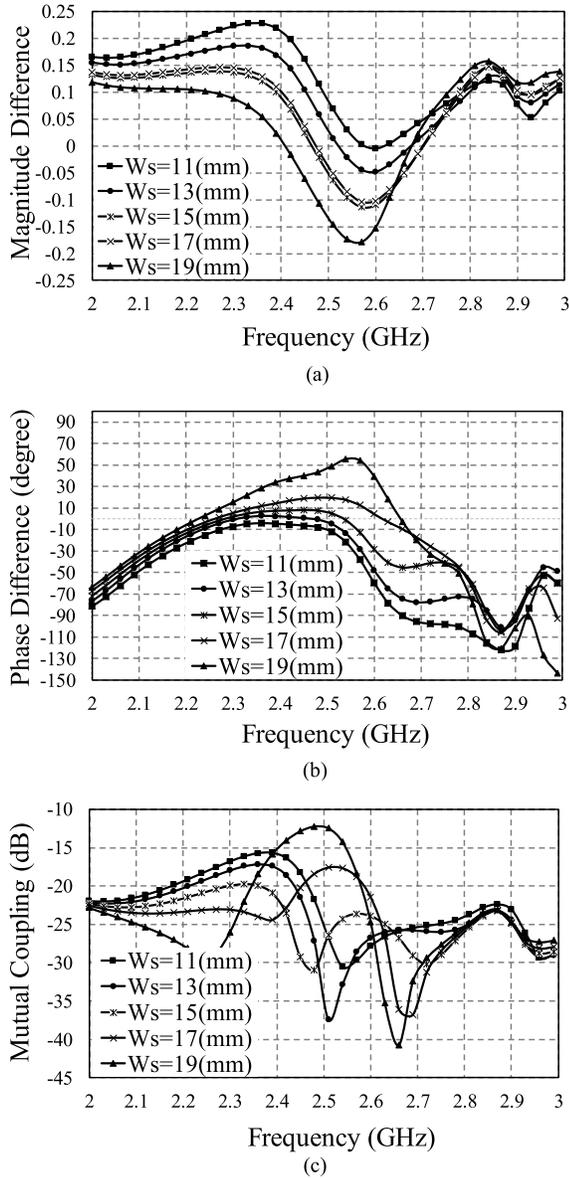
Fig. 5. Simulated (a) magnitude difference, (b) phase difference, and (c) mutual coupling with different sizes of metal strip and  $h = 38$  mm.
