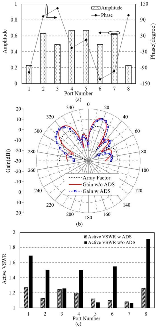
Fig. 10. (a) Weighting coefficients of the eight-element phased array. (b) Synthesized AF and the active radiation patterns of the array with and without the ADS. (c) Largest active VSWR at each antenna port with and without the ADS when the weighting coefficients are applied to the array.
