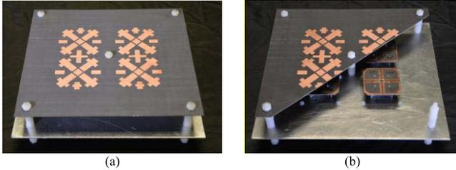
Fig. 13. Photograph of the prototype of the 2 by 2 dipole array antenna with the ADS. (a) Array with the ADS on top. (b) Array with the ADS half cutoff.
