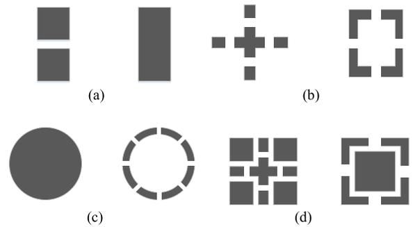
Fig. 2. Some geometries of metal reflection patches. (a) Patches for linearly polarized antennas. (b) Patches for dual-polarized antennas. (c) Patches for circularly polarized antennas. (d) Some composite patches.
