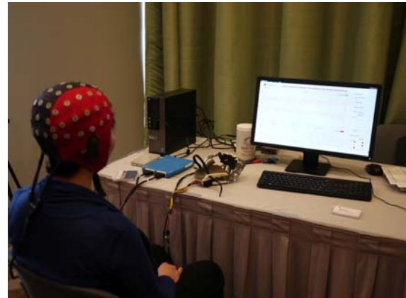
The EEG and hand exoskeleton robot system for stroke rehabilitation
