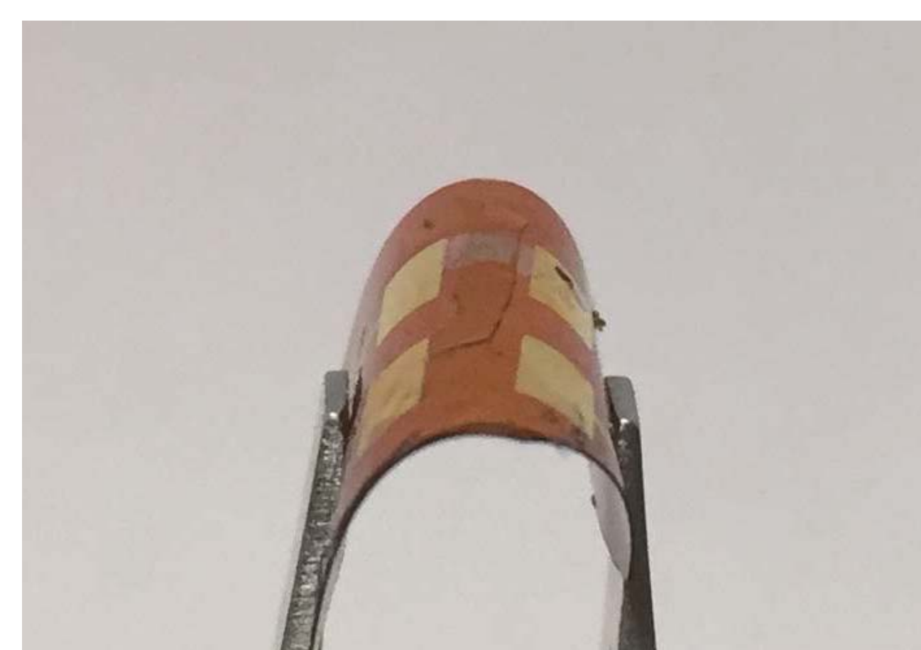
Fig. 3.2 Flexible feature of the transistor
