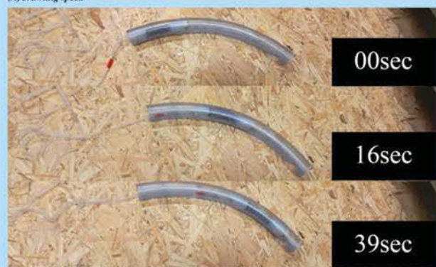
Fig.A shows the robot crawling in a PVC tube, it finish a 20cm crawling in 40 sec. The speed of crawling is 0.5cm/sec.
