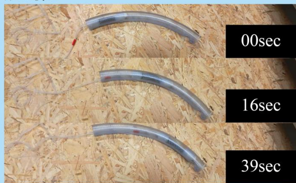
Fig.A shows the robot crawling in a PVC tube, it finish a 20cm crawling in 40 sec. The speed of crawling is 0.5cm/sec. Fig.B shows the robot can bend from 0 degree to 340 degree by appying pressure from 4kpa to 52kpa.
