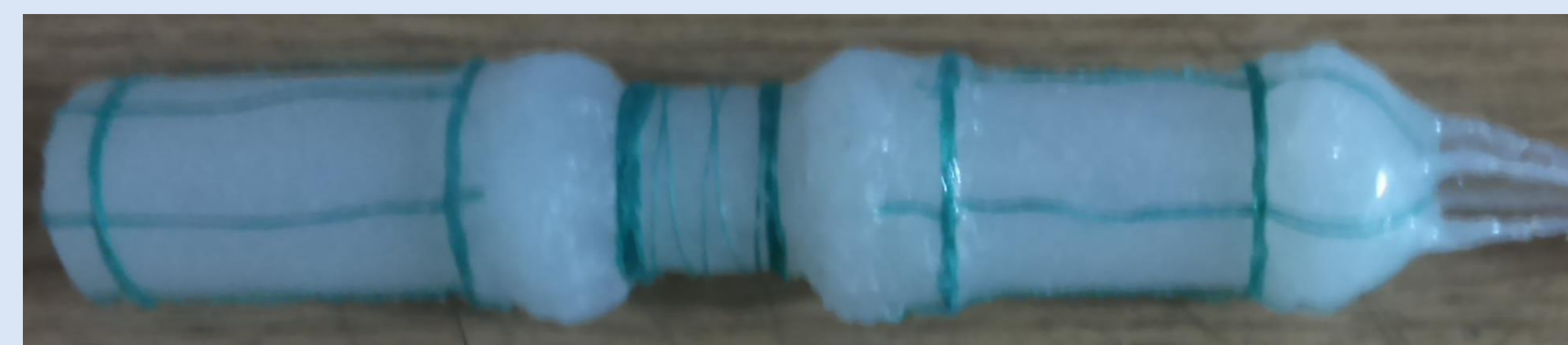
Fig 2. Prototype of the earthworm-like soft robot
