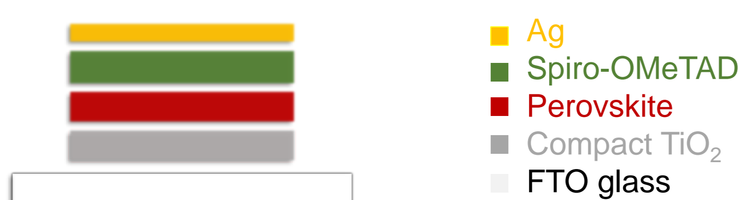
Figure 3. Illustration of a planar solar cell device structure
