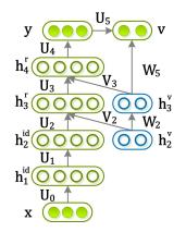
Figure 2: Network structure of MVP, which has six layers, including three layers with only the deterministic neurons (i.e. the layers parameterized by the weights of  $U_0, U_1, U_4$ ), and three layers with both the deterministic and random neurons (i.e. the weights of  $U_2, V_2, W_2, U_3, V_3, U_5, W_5$ ). This structure is used throughout the experiments.
