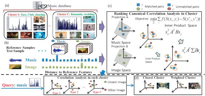
Figure 1: Framework of Multiple Ranking Canonical Correlation Analysis: (a). Cluster in music space; (b). DtRT representation for music and image; (c). Ranking canonical correlation analysis in cluster; (d). Combination of estimation score of clusters.
