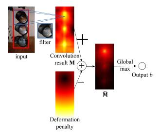
Figure 6. The deformation layer when deformation map is defined in (3). Part detection map  $\mathbf{M}$  and deformation constraint are summed up to obtain the summed map  $\tilde{\mathbf{M}}$ . Global max pooling is then performed on  $\tilde{\mathbf{M}}$  to obtain the score b.
