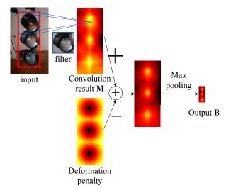
Figure 7. The def-pooling layer. Part detection map and deformation constraint are summed up. Block-wise max pooling is then performed on the summed map to obtain the output  ${\bf B}$  of size  $\frac{H}{k_{tr}} \times \frac{V}{k_{rr}}$ .
