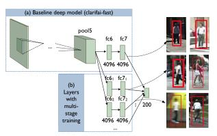
Figure 4. The baseline deep model and fully connected layers with multi-stage training. The layer pool5 is result of max pooling over the conv5 layer in Fig. 3. Different stages of classifiers deal with samples of different difficulty levels.
