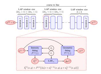
Fig. 3. Registering the source image  $I_2$  to the target image  $I_1$  is performed in a finite number of iterations: the resolution is increased by a factor 2 every three iterations, from a coarse resolution  $n_1 = \min(\text{size of } I_1)/4$  to the fine 1-pixel resolution. An enlargement of a single iteration at resolution  $n_j$  details the sequence of parametric fittings (displacements, intensities) and LAP.
