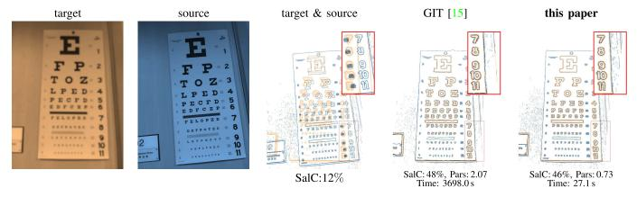
Fig. 9. Registration of real images ( $1440 \times 1080$  pixels) corrupted by blurring, using different algorithms. In order to better visualise the misalignments, we outline them on the feature images. The second row shows the pixel intensity at the 10% largest gradient locations.
