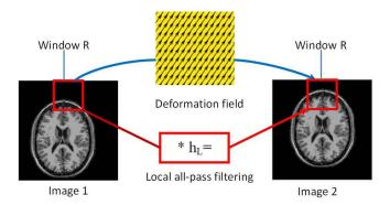
Fig. 2. Illustration of the equivalence between constant displacement field and filtering with an all-pass filter. Note that the locations of the two windows on the right-hand side and left-hand side are exactly the same.
