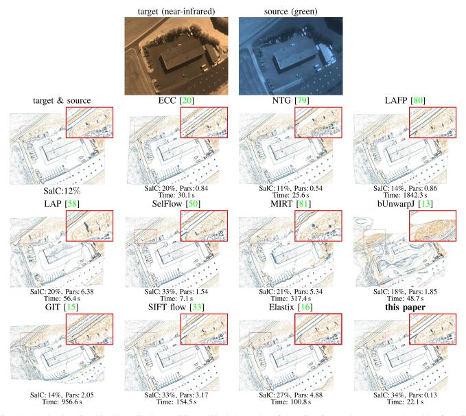
Fig. 11. Registration of multimodal satellite images (960 × 1280 pixels): overlay of the salient features (lower three rows) resulting from different algorithms. The target and source images (top row) are the near-infrared and green channel of a multispectral image taken from the dataset (https://www.sensefly.com/education/datasets/). Our intensity fitting method is histogram matching in this case.
