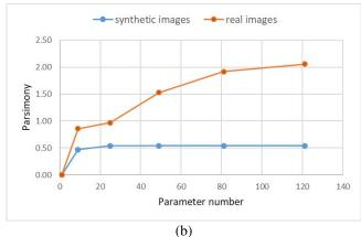
Fig. 12. Increasing the number of Fourier coefficients in the representation of the displacement field, increases the salience correlation (a) and the parsimony (b). The SalC, however, reaches a value larger than 50% quickly and saturates after about 20 parameters. For synthetic images the parsimony saturates quickly at a small value, whereas for real images, it seems to increase without limit, but without significant SalC increase. Images used: same as Fig. 7 (noiseless) and Fig. 8.
