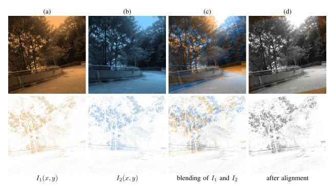
Fig. 1. Top row: the target image (a, orange-toned) is related to the source image (b, blue-toned) through a geometric transformation according to Equation (1) or (2). Blending these images (c) outlines their mis-alignment. Perfect alignment (d) is achieved when the blended image is tone-neutral (i.e., gray). Bottom row: the intensities of the same images at the 10% largest gradient values (visualization better adapted to multimodal images).
