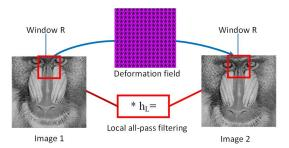
**Fig. 2**. Diagram illustrating the equivalence of constant deformation field and filtering with an all-pass filter in a window. The symbol \* denotes the convolution operator and  $h_L$  is the local all-pass filter of the window. Note that the locations of the two windows on the right-hand side and left-hand side are exactly the same.
