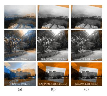
**Fig. 3**. Example of image registration on real images captured by three mobile phones. The images have been downscaled to  $480 \times 640$  (top row),  $1600 \times 1600$  (middle row), and  $960 \times 1280$  (bottom rows). Column (a) shows the source and target image. In column (b), we show the result of methods that perform best in terms of PSNR, with their PSNR and computation time. (c) shows our results.
