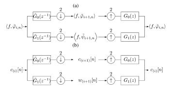
Fig. 4. The discrete wavelet transform for one decomposition level. (a) The continuous-domain representation. (b) The discrete-domain representation.
