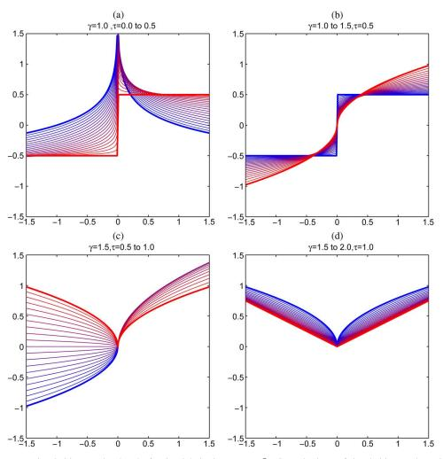
Fig. 1. Family of elementary singularities associated to the fractional derivative operator  $\partial_{\tau}^{\gamma}$ . Several subsets of singularities are shown in (a)–(d). The sweep-through starts in blue and ends in red.
