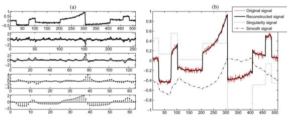
Fig. 9. The SNR improvement of the reconstructed signal is 7 dB (noisy signal 20 dB).
