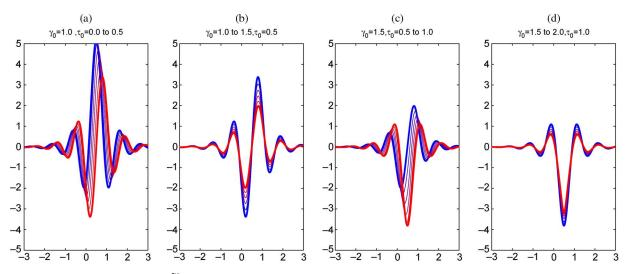
Fig. 5. Effect of the elementary singularity  $\partial_{-\tau_0}^{-\gamma_0}$  on the operator wavelet ( $\gamma = 3, \tau = 0$ ). Several subsets of singularities are shown in (a)–(d). The sweep-through starts in blue and ends in red.
