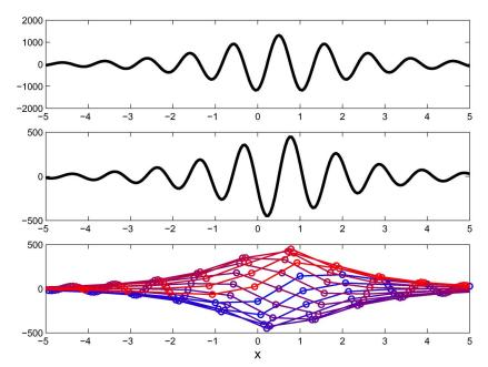
Fig. 6. Mono- or bimodal character of the wavelet coefficients of an edge singularity  $\rho_{0.5}^1(x - x_0)$ , where  $x_0$  varies between 0 and 1 and 14 steps. Top: operator wavelet  $\gamma = 8$ ,  $\tau = 0$ . Middle: operator wavelet acting on edge singularity. Bottom: wavelet coefficients of the edge singularity at different shifts  $x_0$  (red to blue) are sampled versions of the middle plot; they are all mono- or bimodal.
