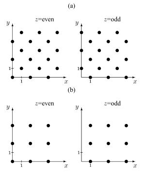
Fig. 2. Two-dimensional cuts of the 3-D lattices obtained by iterating the 3-D FCC dilation. (a) Dk. (b)  $D^2k$ .
