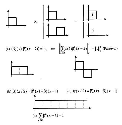
Fig. 2. Illustration of the key properties for the Haar case  $\varphi(x) = \beta_+^0(x)$  (B-spline of degree zero). (a) Orthogonality. (b) Two-scale relation. (c) Wavelet relation. (d) Partition of unity.
