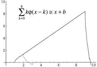
Fig. 5. Illustration of the reproduction of polynomials of degree 0 and 1 using Daubechies scaling functions of order  $\delta=2$ .
