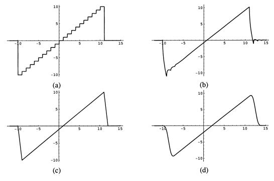
Fig. 4. Plot of  $\sum_{k=-10}^{+10} k \beta_+^{\alpha}(x-k)$  for various values of  $\alpha$ . (a)  $\alpha=0$  (piecewise constant). (b)  $\alpha=0.5$  (fractional spline). (c)  $\alpha=1$  (linear spline). (d)  $\alpha=3$  (cubic spline). This illustrates the property that the B-splines are able to reproduce a first order polynomial as soon as  $\alpha>0$  (i.e., cases b, c, and d, but not a)
