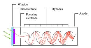
Fig. 7. Schematic representation of a photomultiplier tube (PMT).
