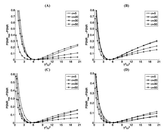
Fig. 5. Sensitivity of our denoising function (14) with respect to variations of T. (a) Peppers 256 × 256. (b) MIT 256 × 256. (c) Lena 512 × 512. (d) Boat 512 × 512. We can notice that for all images and for the whole range of input PSNR the maximum of the PSNR is reached for  $(T^2/\sigma^2) \simeq 6$ .
