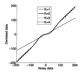
Fig. 4. Shape of our denoising function (12) in a particular subband, for various K and optimized  $a_k$ 's and T.
