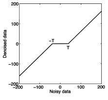
Fig. 2. Soft-thresholding function.
