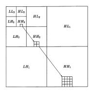
Fig. 6. Three stages of a fully decimated orthogonal wavelet transform and the so-called parent–child relationship.
