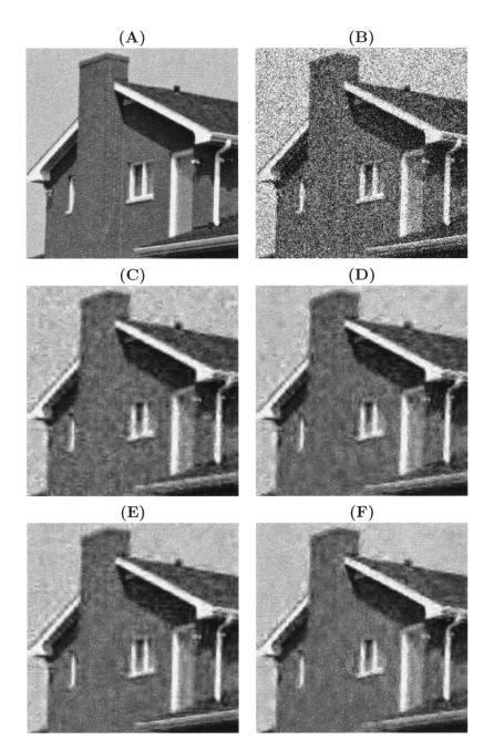
Fig. 12. (a) Part of the noise-free  $256 \times 256$  House image. (b) Noisy version of it: PSNR = 18.59 dB. (c) Denoised result using the *BayesShrink*: PSNR = 27.57 dB. (d) Denoised result using the *BiShrink*  $7 \times 7$ : PSNR = 28.19 dB. (e) Denoised result using the *BLS-GSM*  $3 \times 3$ : PSNR = 28.73 dB. (f) Denoised result using our interscale dependent thresholding function (21): PSNR = 28.96 dB.
