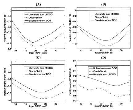
Fig. 11. Comparison of our interscale dependent thresholding function (21) with the best possible soft-threshold *OracleShrink* and with our simple univariate denoising function (14). (a) *Peppers* 256  $\times$  256. (b) *House* 256  $\times$  256. (c) *Lena* 512  $\times$  512. (d) *Barbara* 512  $\times$  512.
