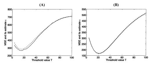
Fig. 3. Statistical accuracy of Theorem 1 illustrated with the *soft-threshold*: true MSE is in dashed lines, while its estimate  $\epsilon$  is in solid line. (a)  $N = 32 \times 32$  samples and  $\sigma = 20$ . (b)  $N = 256 \times 256$  samples and  $\sigma = 20$ . The variance of the estimator decreases when the number of samples N increases, making Theorem 1 statistically reliable for image denoising applications.
