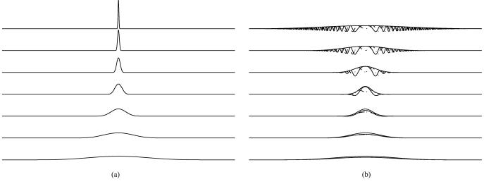
Fig. 2. B-Spline multiresolution and its Fresnel counterpart. (a) B-splines:  $2^{(-j/2)}\beta^3(2^{-j}x)$ , j=-2,-1,0,1,2,3,4. (b) Corresponding F-splines:  $2^{(-j/2)}\bar{\beta}_{2-j}^3(2^{-j}x)$ . In this illustration,  $\tau=0.9$ . The real part is displayed with a continuous, the imaginary part with a dashed line. For the F-splines, we also show the envelopes of the signals.
