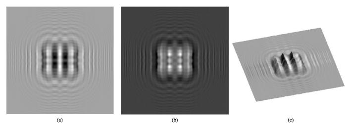
Fig. 4. Propagated target's (a) amplitude and (b) phase. d=30 cm and  $\lambda=632.8$  nm. Sampling step  $T=10~\mu$ m. The sampling step is  $T=10~\mu$ m and  $512\times512$  samples are evaluated. (c) Perspective view.
