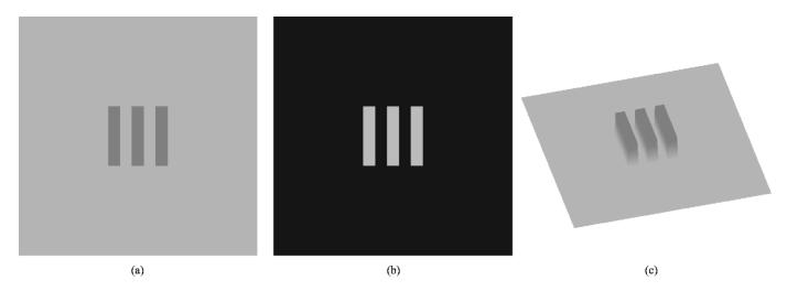
Fig. 3. (a) Amplitude and (b) phase of the test target. The bars width is 256  $\mu$ m. The sampling step is  $T=10~\mu$ m and  $512\times512$  samples are evaluated. The amplitude is equal to 1 (dark grey) or  $\sqrt{2}$  (light grey). The phase is equal to 0 (black) or  $\pi/4$  (light grey). (c) Perspective view. The grayscale is representative for the amplitude and the elevation for the phase.
