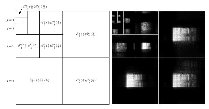
Fig. 9. Fresnelet transform of the modulated hologram R'I (coefficient's amplitude). There are  $2048 \times 2048$  coefficients.
