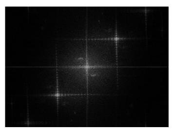
Fig. 8. Absolute value of the Fourier transform of the hologram. The frequency origin is in the center.
