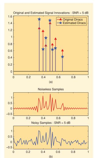
[FIG3] Retrieval of an FRI signal with (a) seven Diracs from (b) 71 noisy (SNR  $=\,$  5 dB) samples.
