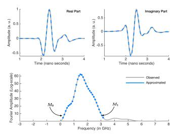
Fig. 3: Approximation of kernel used for ground penetrating radar experiment via finite Fourier series. The measured data is shown in grey ink. Dashed blue lines show its approximated version. Here T = 10.14 ns and  $M_0 = 0.19$  GHz and  $M_1 = 3.15$  GHz.
